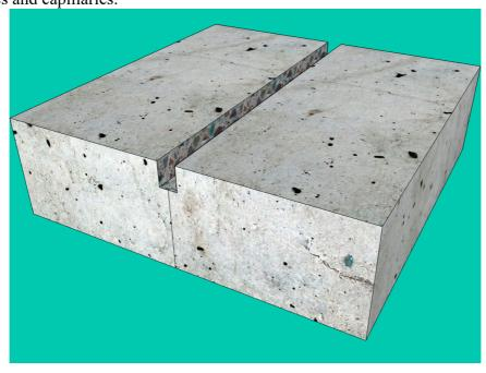
Insure that all cracks are channeled at least 10 cm beyond the visible end of the crack. In areas in which structural reinforcing steel does not allow 3.5 cm consistently, chip or chisel or route the concrete on both sides of the steel to the appropriate depth and clear the area over the steel to whatever depth is allow by the placement of the steel.
