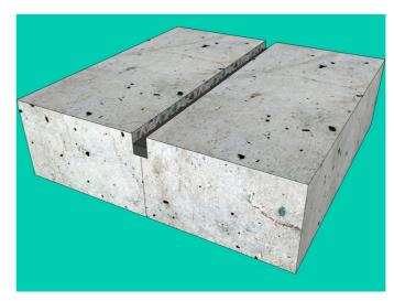
keep firm hand pressure on the repair area until the plug has hardened. Insure that Crystal Stop does not exceed 1/2 of the channel height.
